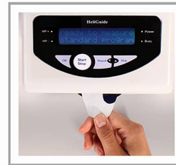
Insert Breathcard into HeliGuide analyzer
